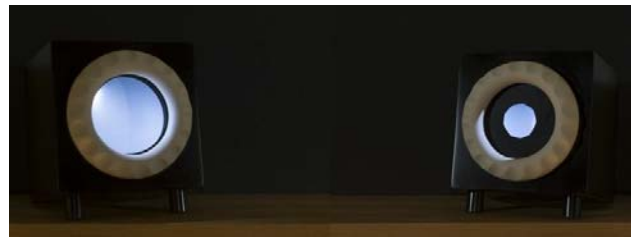
Figure 4: The IrisBox. Left: the owner of this box is available for communication. Right: the aperture is almost closed which indicated a low willingness to communicate.
