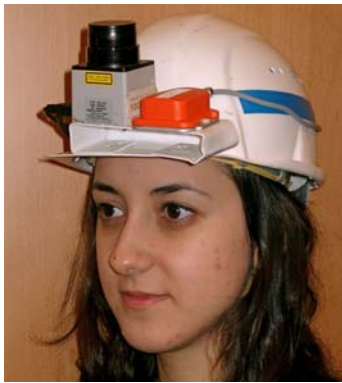
(a) The test person with Hokuyo laser scanner and XSens sensor mounted onto her helmet.
