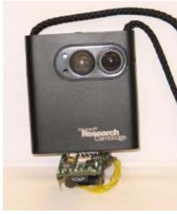
(a) SenseCam with added compass sensor
